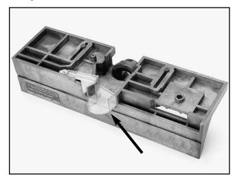
Figure 12. Correctly installed guard.
